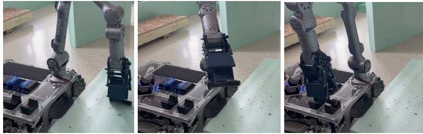
Fig. 8: Three images are shown, from left to right, picking an object, moving towards an object tray, and placing object in object tray.
